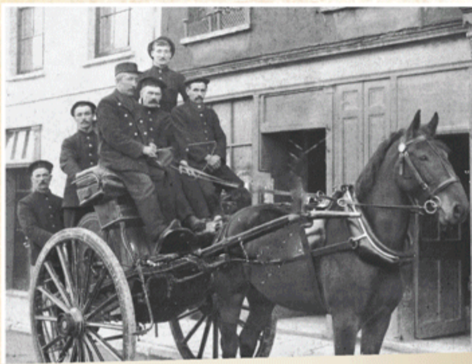
As late as 1920, Cork Fire Brigade crews relied mostly on horse-drawn 'jumper' appliances like this one photographed in 1906. Firemen connected a hose reel beneath the carriage to street hydrants.
